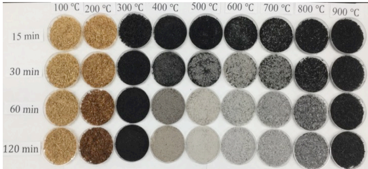
Fig. 2-2-2. Appearance of the rice husk ash after different calcination temperatures and durations
